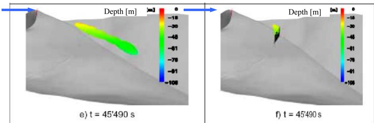
Fig. 9 Comparison of the vertical velocity field without (left) and with the diaphragm (right) in the delta region. The current is almost completely blocked by the obstacle during the flood event.
