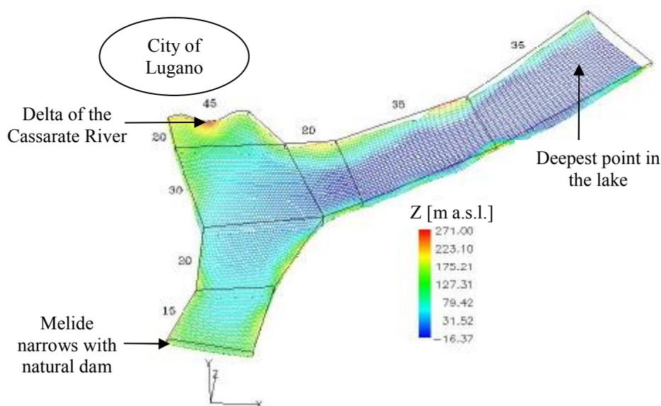
Fig. 5 Structured grid of the lake bottom of the North Basin with a total of 195'750 cells, distributed over seven blocks used for the numerical model
