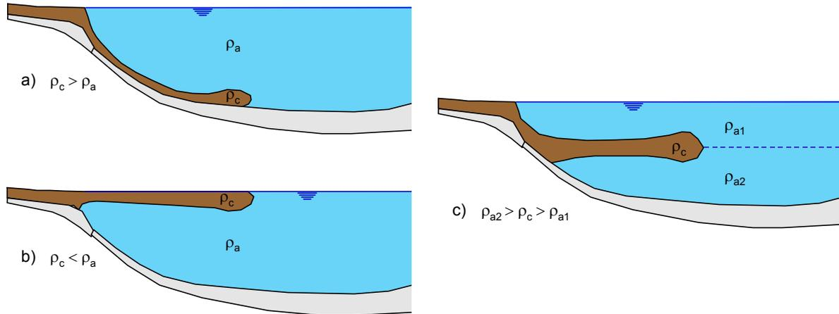
Fig. 1 Density currents of density  $\rho_c$  in a non-stratified lake of density  $\rho_a$  and in a stratified domain of density  $\rho_{a1}$  respectively  $\rho_{a2}$  in the form of a) underflow b) overflow and c) interflow (De Cesare 1998)
