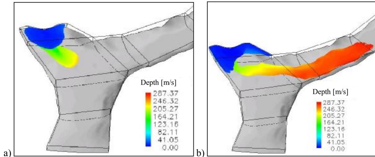
Fig. 7 Bottom density current (underflow) and intrusive current (interflow), global view with surface of equal concentration coloured according to depth, three hours (a) and in its final position nine hours (b) after the 1999 flood peak
