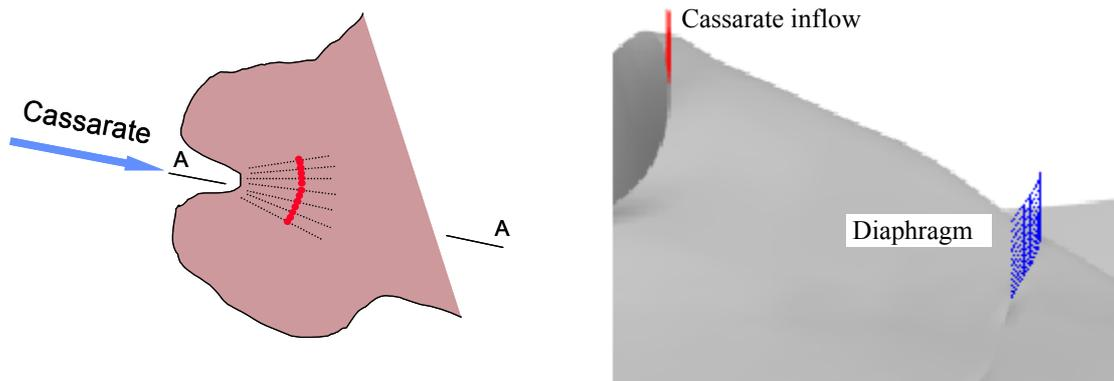
Fig. 8 Situation with axes A-A (left) and lateral view of the vertical diaphragm in the numerical model (right)
