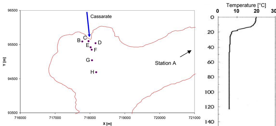
Fig. 4 Measuring stations close to the Cassarate mouth (operated by LSA); Station A is close to the deepest point in the lake (see Fig. 5). Measured temperature distribution at station F in September 1999.
