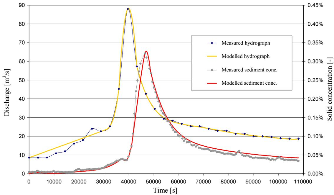
Fig. 3 1999 flood hydrograph and evolution of the sediment concentration in the Cassarate River, observed and modelled values
