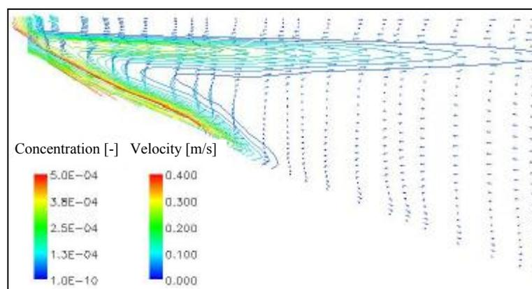
Fig. 6 Bottom density current (underflow) and intrusive current (interflow) as lines of equal concentration and velocity vectors in the axial longitudinal plane, one hour after the 1999 flood peak
